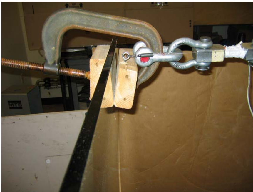
Fig. 4 - Initially, a single C-clamp was used, but the clamp bent during testing as shown. Two clamps had to be used for the remaining tests.
