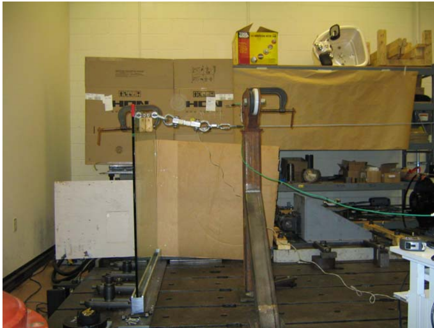
Fig. 1 - An overall view of the first test setup is shown. The load was applied at the center of the top edge of the glass panel. Wood blocks were used to distribute the clamping pressure and prevent fracture of the glass.
