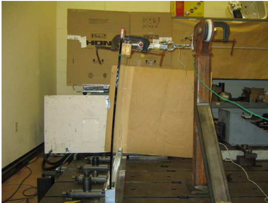
Fig. 3 - The deflected glass panel is shown with 550 pounds (2,446 N) applied.
